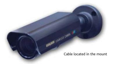
This 1/4" color CCD camera, has a 4mm-9mm adjustable varifocal lens and electronic shutter to give the perfect picture in a wide variety of installations. The weather-resistant housing is furnished with a protective sunshield and the cable is routed through the "conduit compatible" mounting bracket for extra protection.
